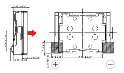
Positive voltage on pin '+' moves membrane in direction of red arrow!
